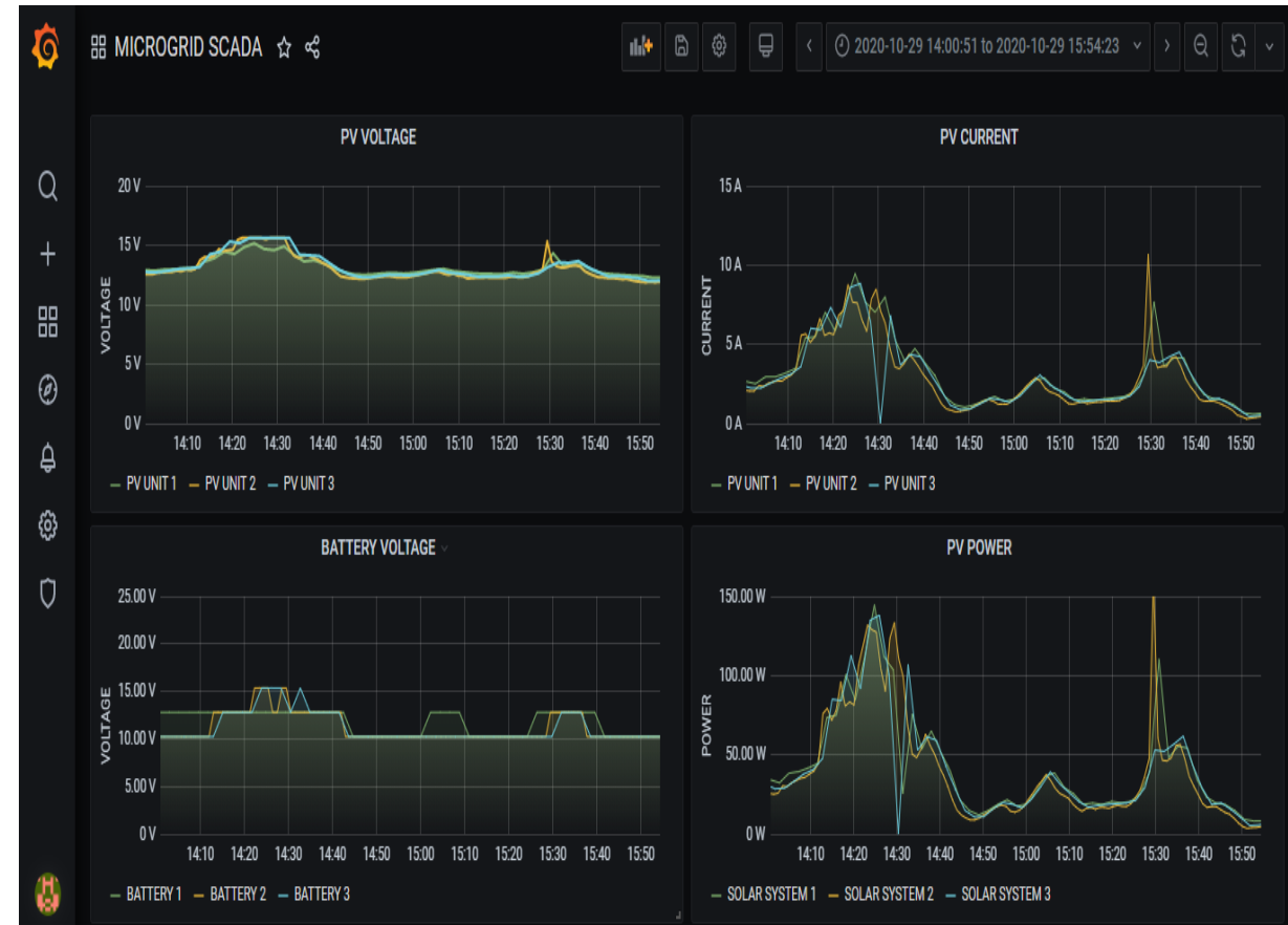
Fig. 53. Real-time data measurement displayed on Grafana dashboard.
