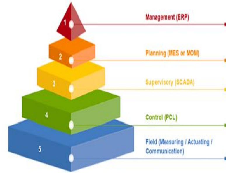
Fig. 41. Industrial automation Pyramid
