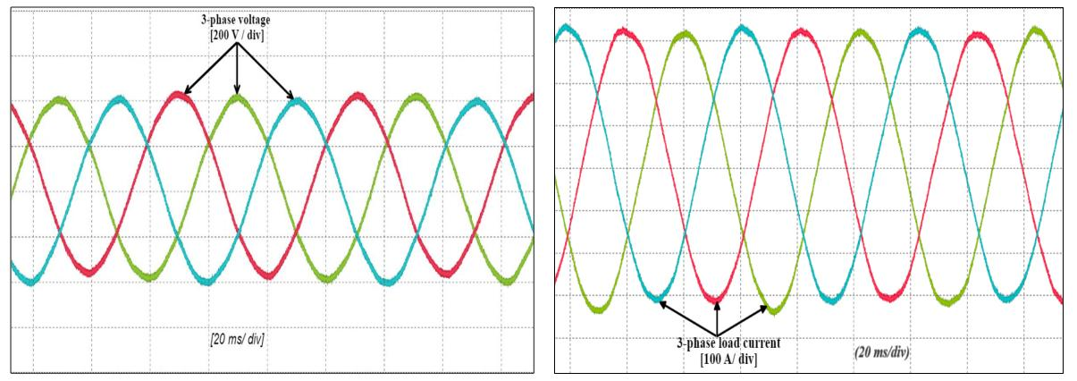
Three-phase output load voltage
