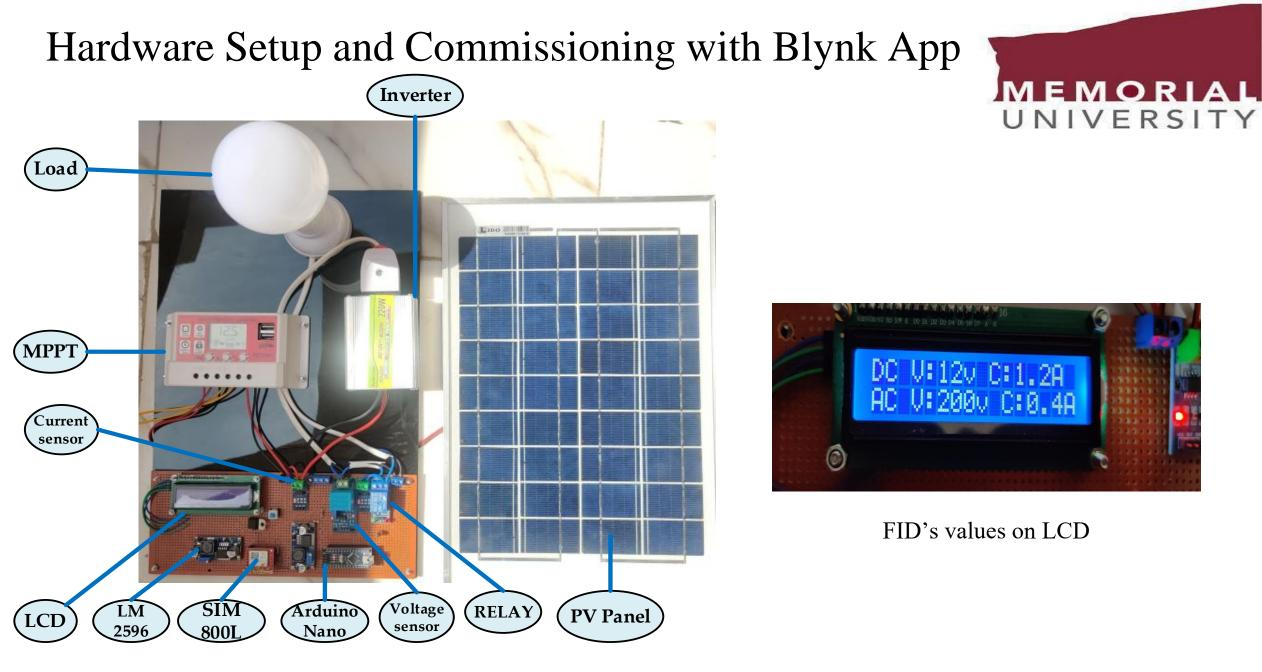
Hardware setup using GSM and Arduino Nano
