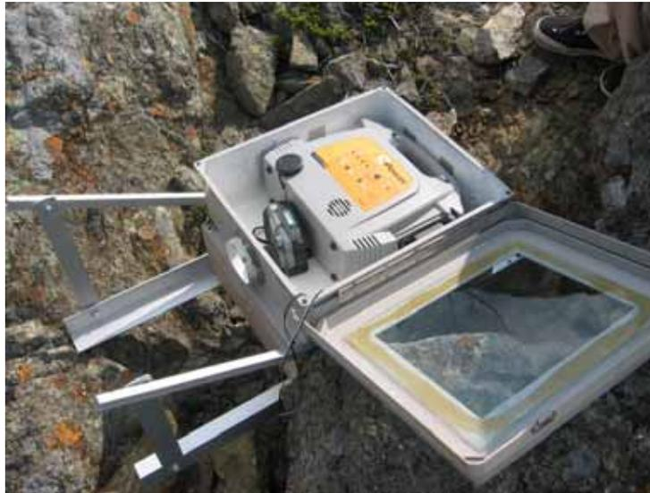
**Figure 2.1 Remote camera system with Kodak DC290.**
