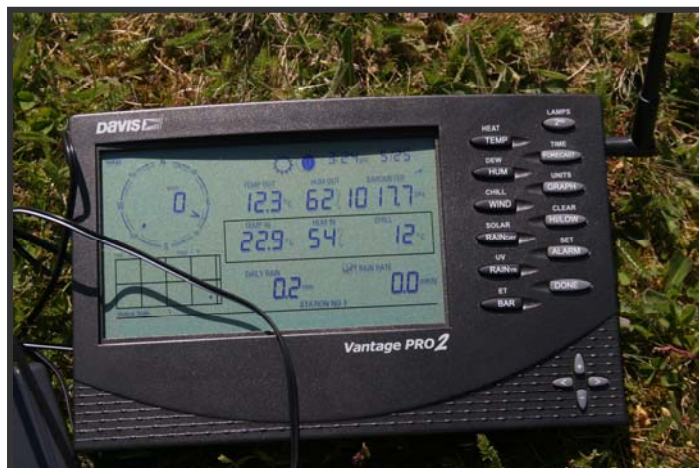
Meteorological Station Components Left = Weather Instruments Above = Data Display and Logging Unit
