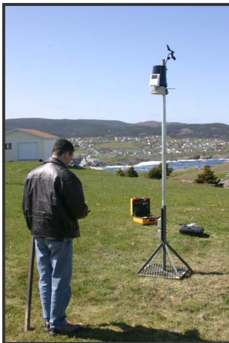
Meteorological Station Components Left = Weather Instruments Above = Data Display and Logging Unit
