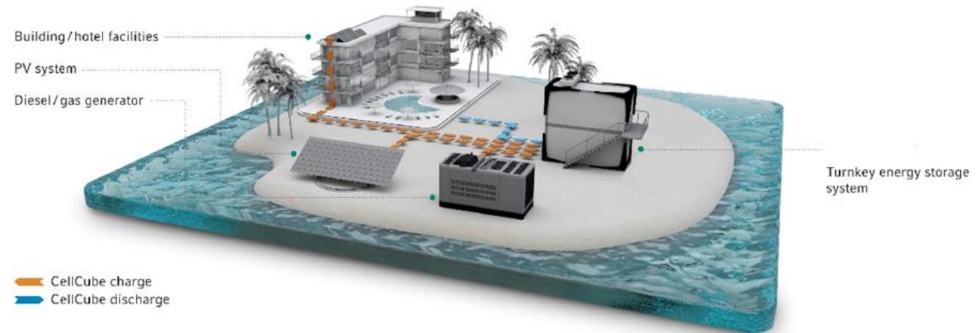
Figure 4. A Graphic of an Isolated Hybrid Power System
