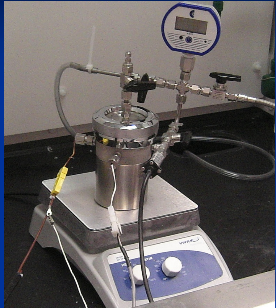
The picture of ARSST standard containment vessel
