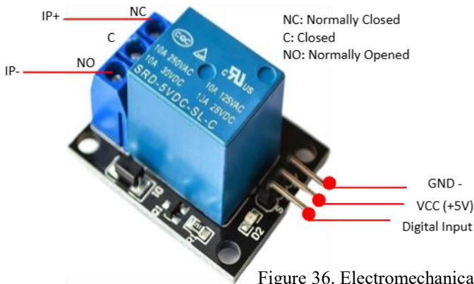
Figure 36. Electromechanical Relay Module.
