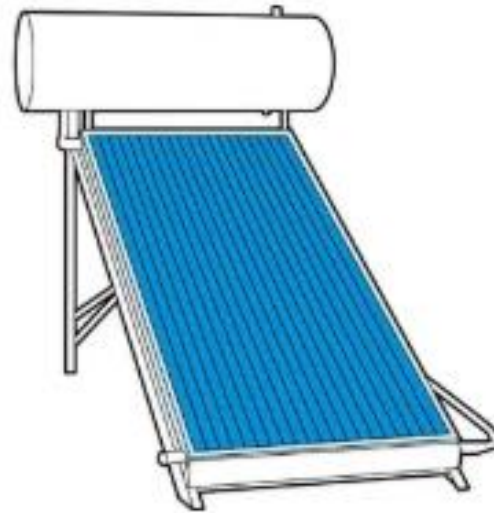
Fig. 3 Flat plat collector (water-based)
