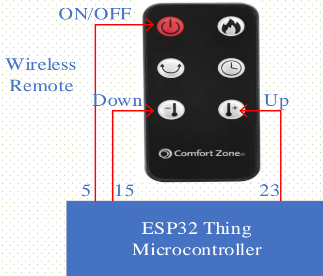
Connection diagram of remote and ESP32 Thing
